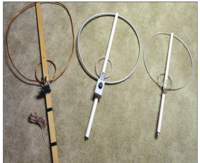
Figure 2 — Tracking loop antennas. Left to right: 24-inch copper loop, 20-inch aluminum loop, 16-inch #22 AWG wire loop with plastic tubing.
